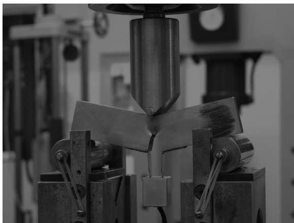
FIG. 1 Fracture toughness test for a precracked specimen, material B.
