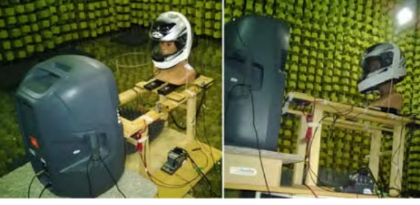
Fig. 9 Experimental setup in the anechoic room.
