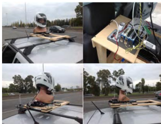
Fig. 4 Experimental setup on and inside the car during the freeway experience.
