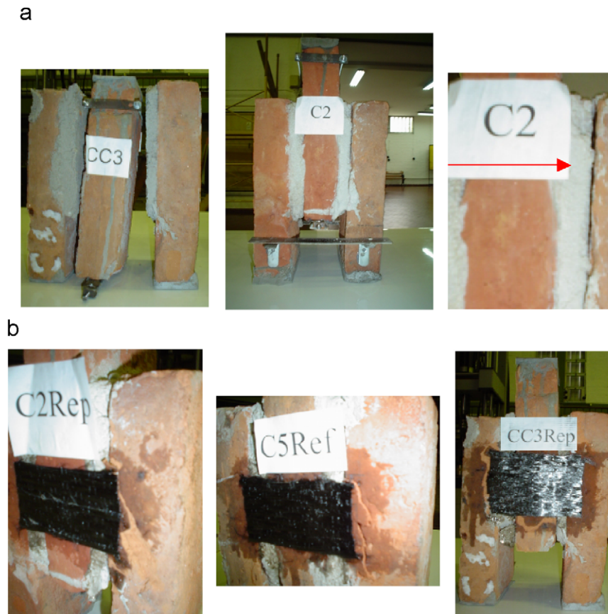
Fig. 5. Failure modes for tested triplets: (a) unreinforced specimens; (b) repaired and retrofitted specimens.
