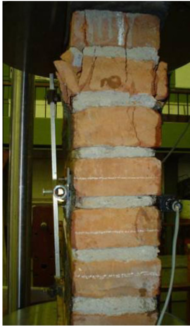
Fig. 11. Compression normal to the bed joint of CFRP repaired specimens. Failure mode.
