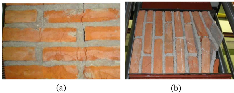
Fig. 6. Compression test failure pattern. (a) Normal to the bed joint (MN1, MN2, MN3, MN6, MN7). (b) Parallel to the bed joint (MP1, MP2, MP3).
