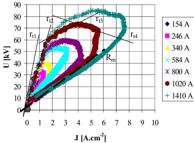
**Figure 4.** Characteristics voltage/current density for  $\sigma=2.8 \text{ mS m}^{-1}$ . Current crest value  $I_{\max}$  as parameter, derivative of transient resistances  $r_{ti}$  at different times  $t_i$  ( $i = 1 \dots 4$ ).
