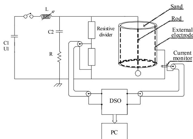
Figure 1. Test circuit and cylindrical cell.
