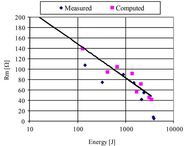
**Figure 10.** Measured and computed minimal transient resistance as a function of injected energy (negative polarity). See Table 1.
