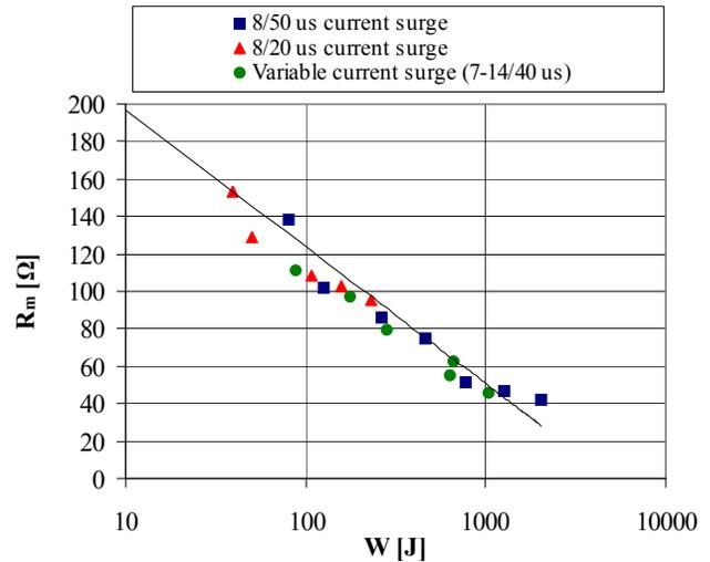
**Figure 5.** Measured minimal transient resistance as a function of injected energy (both polarities).
