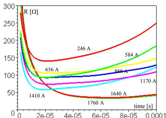
**Figure 8.** Computed transient resistances for the cases of Table 1.
