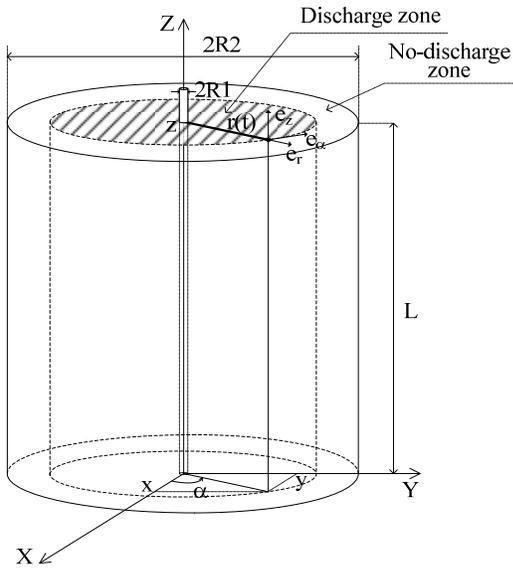
Figure 6. Ionized region into the test cell.
