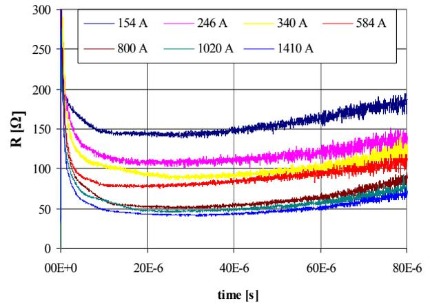
**Figure 3.** Resistance as a function of time for several current densities, with ionization (10/40 μs current surge).
