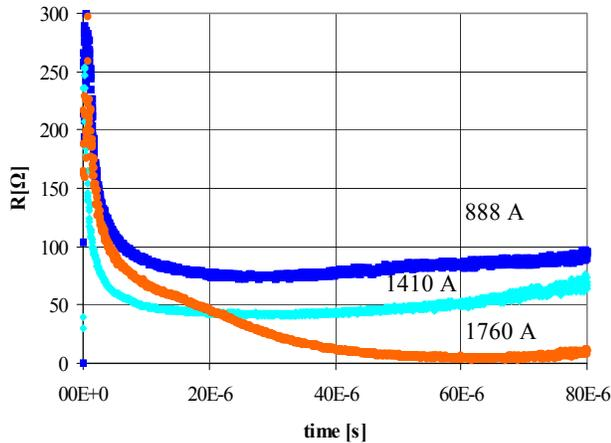
**Figure 9.** Measured transient resistances for three current waveforms: 10/40  $\mu\text{s}$  (1410 A), 15/50  $\mu\text{s}$  (888 A), 40/70  $\mu\text{s}$  (1760 A). See Table 1.
