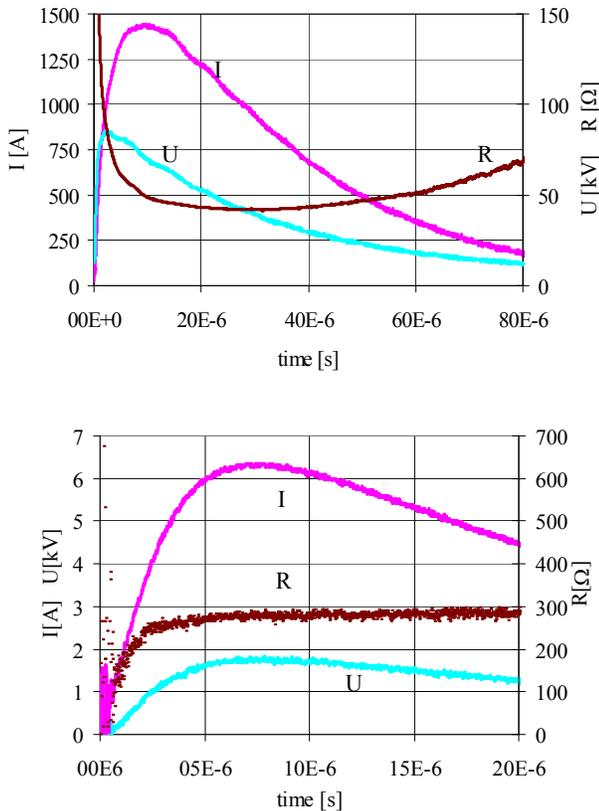
**Figure 2.** Current, voltage and resistance as a function of time. Without ( $I_{max}=6.4$  A) and with ionization ( $I_{max}=1410$  A).
