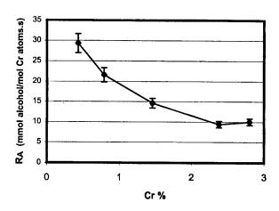
Fig. 1. Ethanol dehydrogenation over  $Cr/SiO_2$  catalysts at different chromium contents. 5 KPa of alcohol and 593 K
