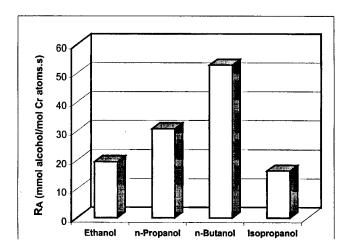
Fig. 2. Oxydehydrogenation of different alcohols on 1.46% Cr/SiO<sub>2</sub>. 5 kPa of alcohol, 2.2 kPa of O<sub>2</sub> and 538 K
