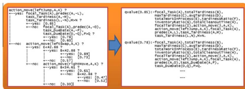
Fig. 4. A simple example of a relational regression tree (left), and a detail of two from ten possible derived Prolog rules (right).
