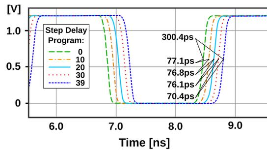
Fig. 9 Timing simulation result of the wide range delay cell with different programmed delay
