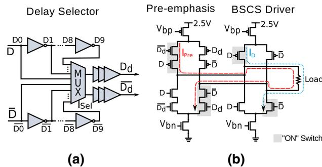
**Fig. 13** BSCS driver with programmable pre-emphasis circuit: **a** pre-emphasis delay selector, **b** BSCS driver with pre-emphasis circuit
