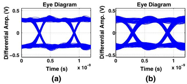
**Fig. 20** Eye diagrams output at 1.66 Gb/s: **a** with *minimum* amount of pre-emphasis and after 6'' FR4 copper channel model and **b** *medium* amount of pre-emphasis and after 30'' FR4 copper channel model
