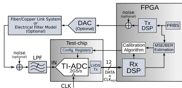
**Fig. 2** Complete platform concept for evaluation of mixed-signal calibration techniques of time-interleaved ADC
