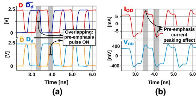
**Fig. 14** Driver signals: **a** driver and pre-emphasis CMOS level inputs ( $D, \overline{D}_d$  and  $\overline{D}, D_d$ ), **b** differential driver current ( $I_{OD}$ ) and differential output voltage ( $V_{OD}$ )
