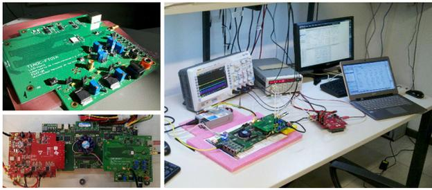
**Fig. 17** A/D converter test board (top-left), FPGA+ADC board (bottom-left), Lab. test setup (right)
