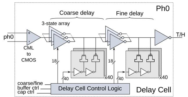
Fig. 8 Programmable delay-cell (Ph0 cell)
