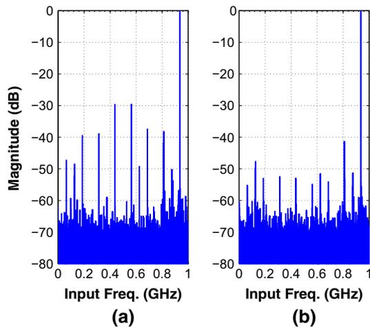
**Fig. 22** FFT Analysis comparison of TI-ADC output: **a** without phase calibration **b** with calibrated phase mismatch using programmable delay cells. Measured at  $V_{INppDiff} = 400$  mV,  $F_{in} = 937$  MHz,  $F_s = 2$  GHz,  $FFT_{samples} = 32768$
