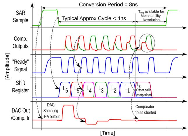
Fig. 11 Asynchronous SAR ADC timing diagram
