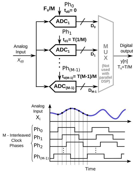
**Fig. 1** Time-interleaved A/D converter
