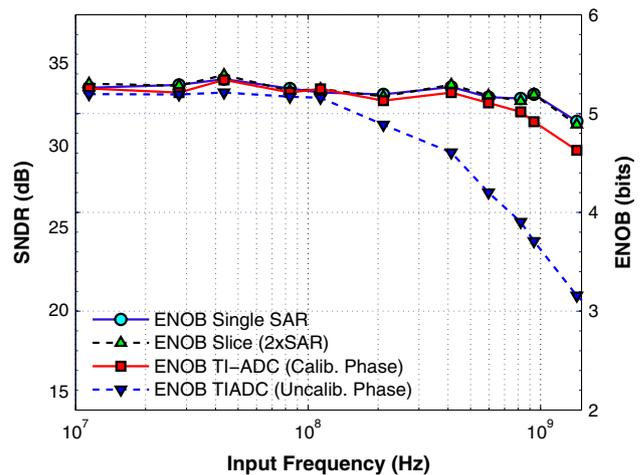
**Fig. 21** SNDR and ENOB versus input frequency
