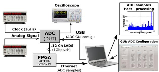
**Fig. 16** A/D converter test setup
