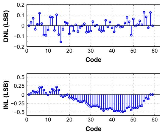
**Fig. 23** Dynamic measurement of DNL and INL for the complete TI-ADC  $F_s = 2$  GS/s,  $F_{in} = 3$  MHz
