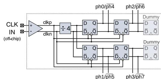
**Fig. 6** 8-Phase generator: CML based double shift register phase generator
