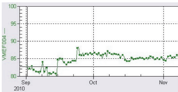
Figure 5. Example of a boiler efficiency trend.
