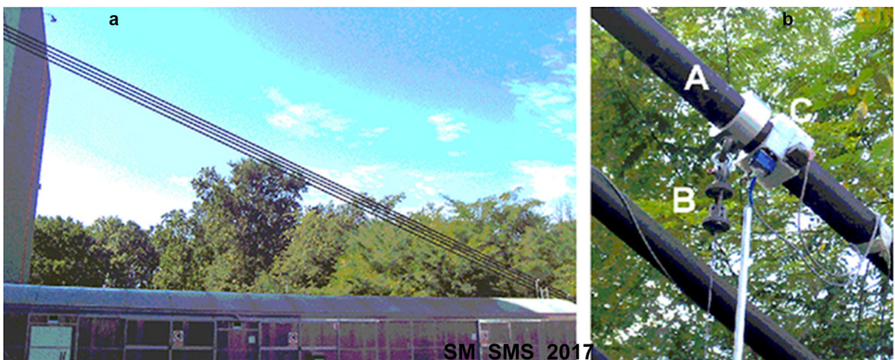
Fig. 4 a ELSA cables 1–2–3–4. b Connections. A Cable No 1. B SMA wire link. C “Rigid” bar transmitting the cable position to the LVDT situated in the bottom
