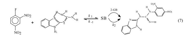
**Table 3.** Reaction of 2,4-dinitrofluorobenzene, DNFB, with histamine, N-(3-amino-1-propyl)morpholine, (3-APMo) and 2-guanidinobenzimidazol, 2-GB, in toluene at  $40.0 \pm 0.2^{\circ}C^{\circ}$  and  $25.0 \pm 0.2^{\circ}C^{\circ}$ , respectively. Second,  $k_A$ , order rate coefficients.
