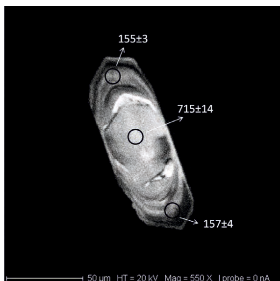
Fig. 2– Cathodoluminescence (CL) image of one zircon from the studied sample. Oscillatory zoning and Proterozoic core are shown.
