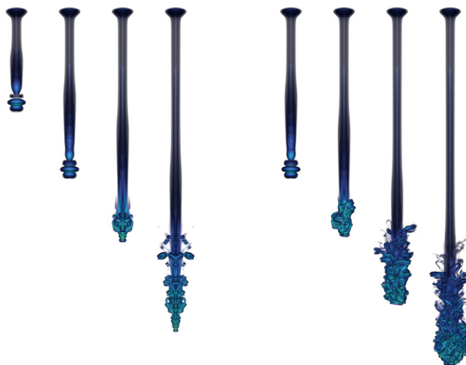
Figure 7. Time series of volume renderings of the enstrophy of a 3D compressible starting plume. Simulation parameters are nearly identical (see text) to those used in the 2D study illustrated by figure 6, yet the behaviour is dramatically different. The background through which the plume is descending is quiescent in the simulation illustrated by the time series on the left and is seeded with low amplitude temperature fluctuations in that illustrated by the series on the right. Rather than pinch detachment of the leading vortex ring, down flowing fluid from behind passes through the vortex torus core and disrupts it.
