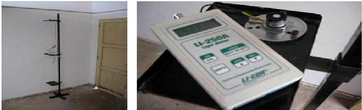
Figure 3: Equipment; Column with pre-fixed heights and LI-210 SB photometric sensor.
