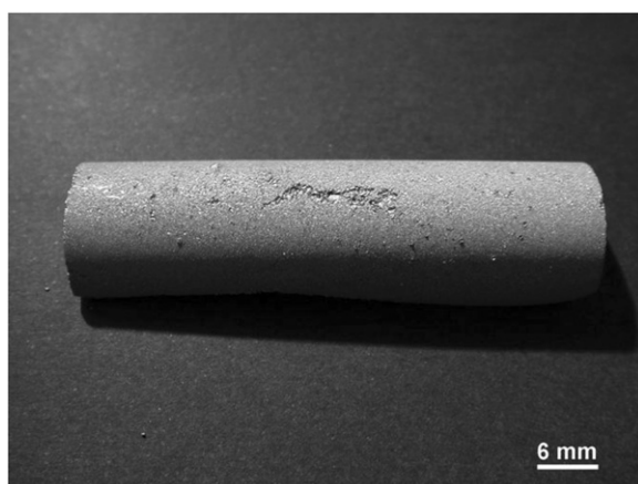
Figure 3. Dehydrided titanium powder slightly sintered during the dehydriding process.
