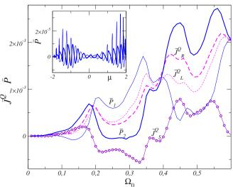
FIG. 4. (Color online) Main panel: Heat currents  $\overline{J}_L^Q, \overline{J}_R^Q$  (dashed thin and thick lines, respectively) and  $\overline{J}_S^Q$  (circles) along the left and right leads and the central system, respectively, for  $\mu$ =-1.5. Powers developed by the external fields  $\overline{P}_1, \overline{P}_2$  (thin and thick solid lines, respectively). Inset:  $\overline{P}_1, \overline{P}_2$  as function of  $\mu$  for  $\Omega_0$ =0.01. Parameters are as in Fig. 2.
