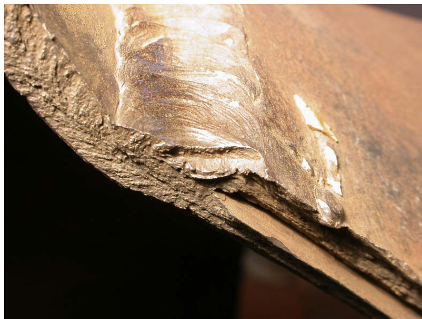
Fig. 8. Brittle fracture with chevron marks in the collector material.
