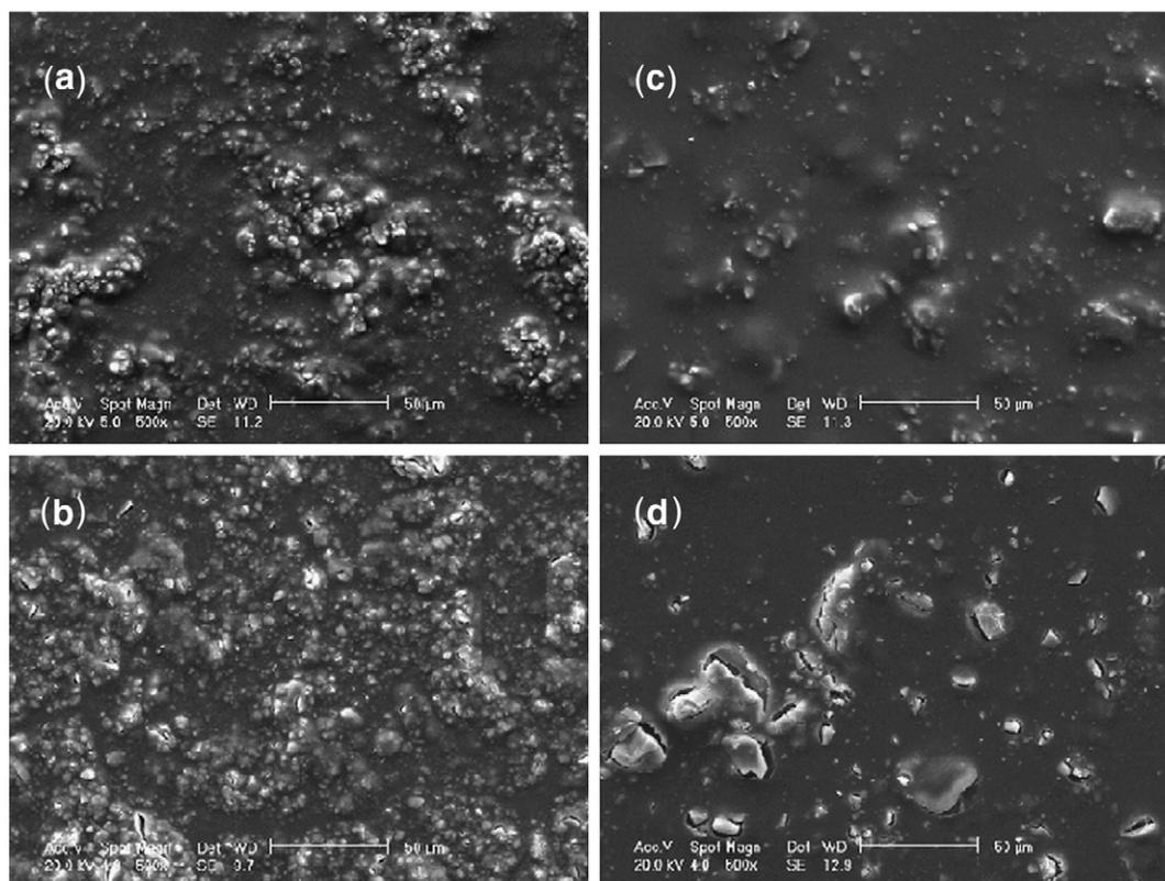
**Fig. 9.** Scanning Electron Microscopy of TEOS–MTES/TMH coated samples with small particles after 1 (a) and 30 days (b) of immersion, and samples with big particles after 1 (c) and 30 days (d) of immersion in SBF at 37 °C.
