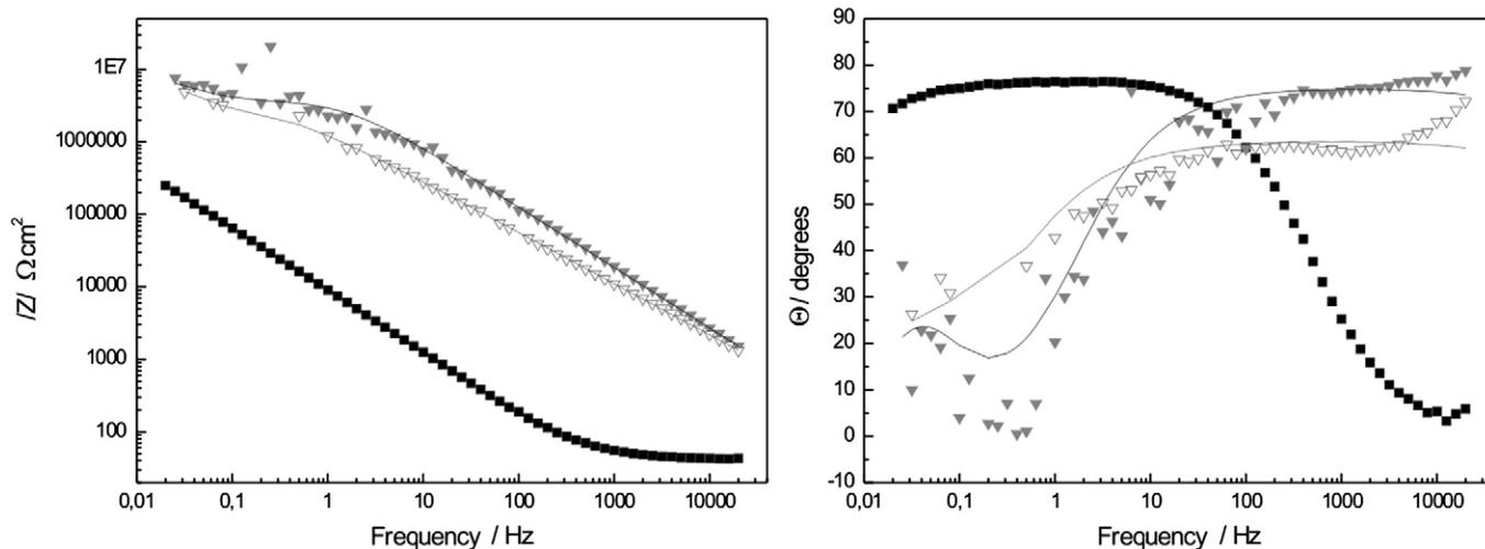
Fig. 7. Bode plots for the TEOS-MTES+TMH coating containing big particles after 1 (▼) and 30 (▽) days of immersion in SBF and their comparison with the bare alloy (■).
