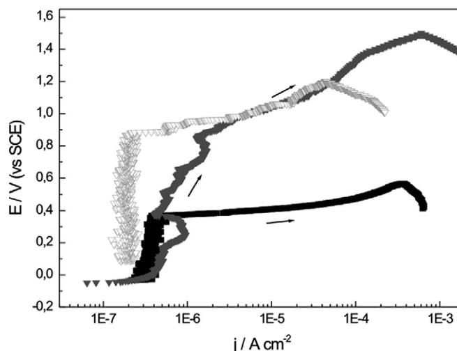
**Fig. 3.** Potentiodynamic polarization curve of the TEOS–MTES / TMH coating containing big particles after 1 ( $\blacktriangledown$ ) and 30 ( $\blacktriangle$ ) days of immersion in SBF, and their comparison with the bare alloy ( $\blacksquare$ ).
