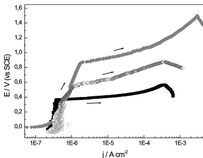
**Fig. 2.** Potentiodynamic polarization curve of the TEOS–MTES+TMH coating containing small particles after 1 ( $\blacklozenge$ ) and 30 ( $\blacktriangledown$ ) days of immersion in SBF and their comparison with the bare alloy ( $\blacksquare$ ).
