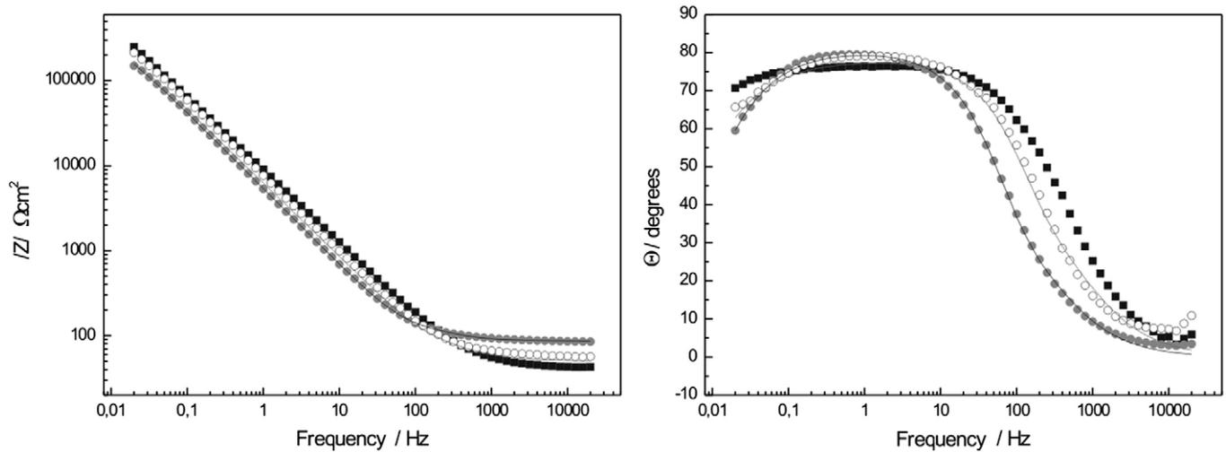
Fig. 4. Bode plots for the TMH coating containing small particles after 1 (●) and 30 (○) days of immersion in SBF and their comparison with the bare alloy (■).
