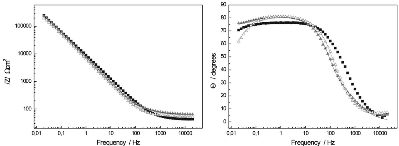
Fig. 5. Bode plots for the TMH coating containing big particles after 1 (▲) and 30 (△) days of immersion in SBF and their comparison with the bare alloy (■).
