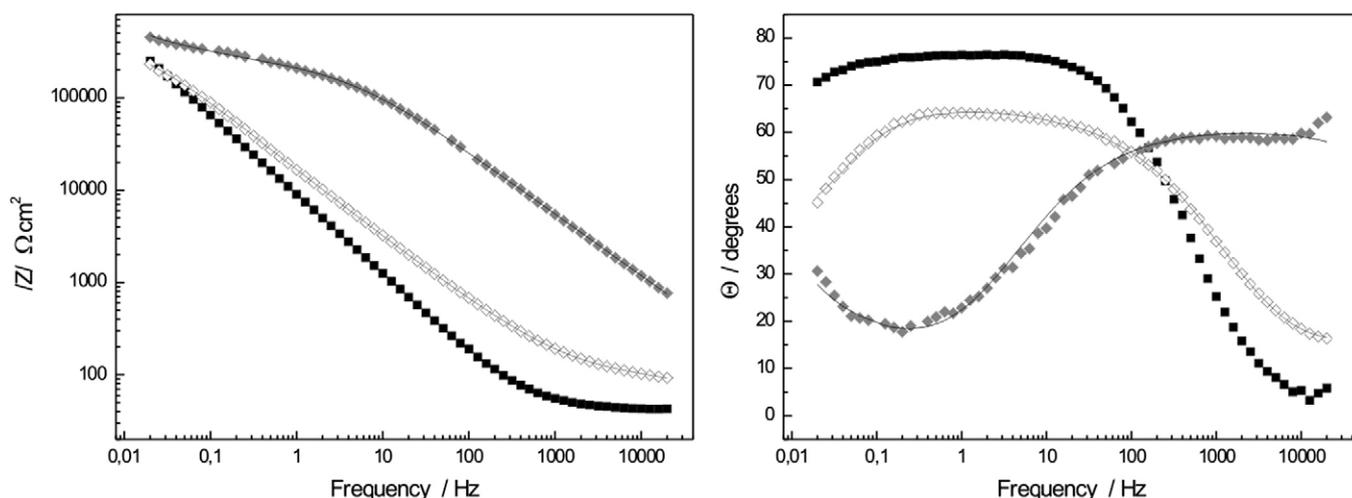
Fig. 6. Bode plots for the TEOS-MTES+TMH coating containing small particles after 1 (◆) and 30 (◇) days of immersion in SBF and their comparison with the bare alloy (■).
