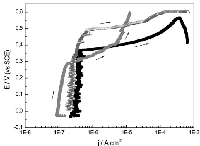
**Fig. 1.** Potentiodynamic polarization curve of the TMH coating containing big particles after 1 ( $\blacktriangle$ ) and 30 ( $\blacktriangledown$ ) days of immersion in SBF and their comparison with the bare alloy ( $\blacksquare$ ).
