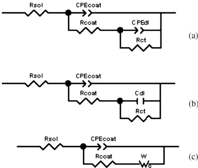
Fig. 8. Equivalent electric circuits employed to model the impedance data of the different coatings after 1 and 30 days of immersion in SBF.
