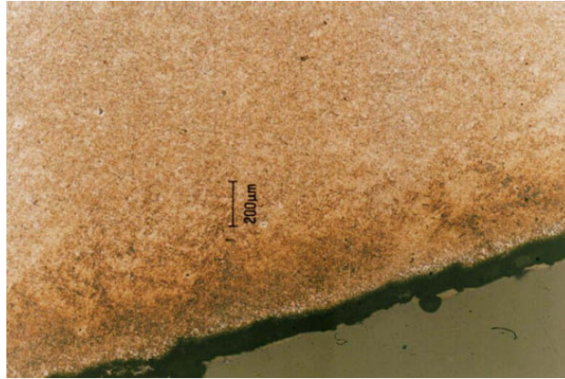
Fig. 8. ( \times 50 ) Microstructure near the failed section, inner pipe surface of pipe wall.
