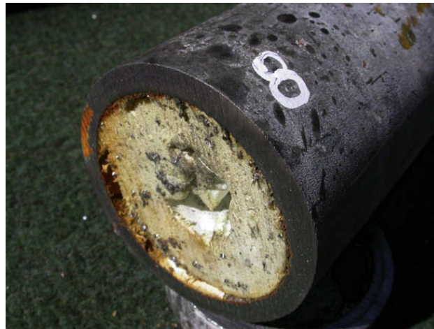
Fig. 4. Not carbonized polymer clog away from the failed section.
