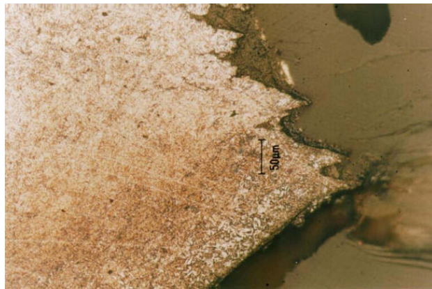
Fig. 9. ( \times 200 ) Crack that led to gas leakage and fire.
