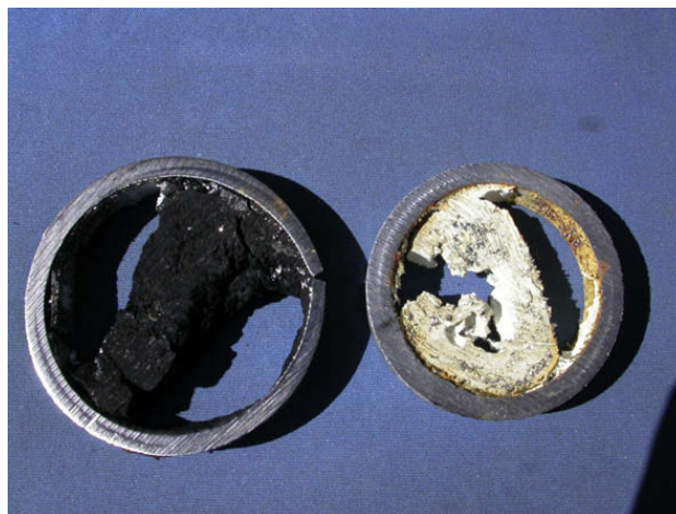
Fig. 5. Sections where polymer residue is thinner.
