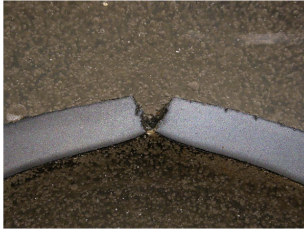
Fig. 6. Polished and Nital etched circumferential specimen.
