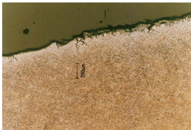
Fig. 7. ( \times 50 ) Microstructure near the failed section, outer pipe surface of pipe wall.
