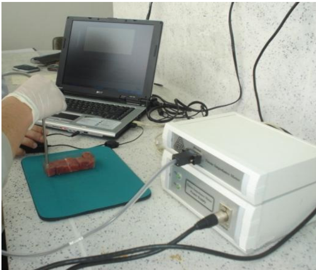
Figure 4. Electrical impedance spectroscopy MK3.5 single channel system.
