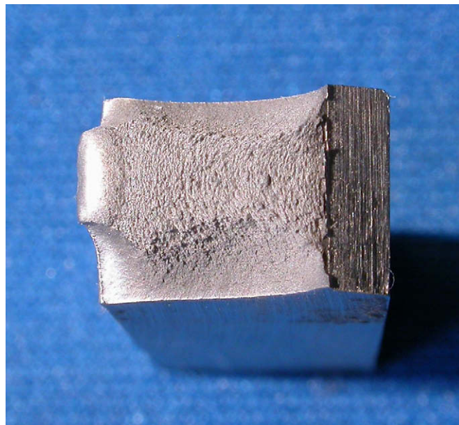
Fig. 6. Fracture surface of a specimen from a cracked curve.
