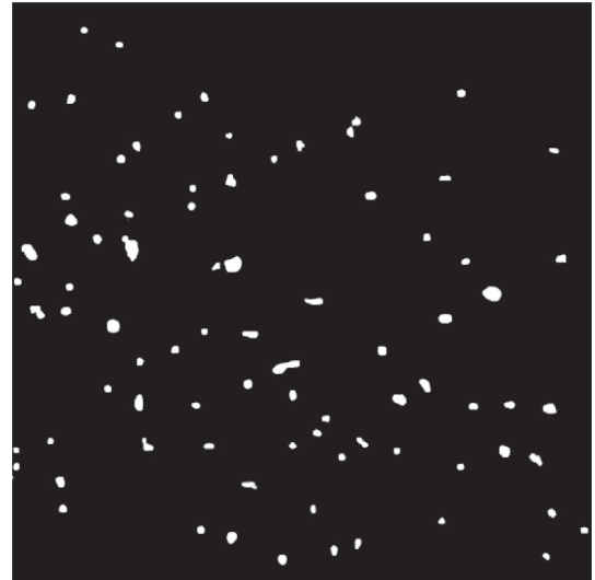
Fig. 3. Processed binary image containing carbides with a mean diameter larger than 0.33 \mu\text{m} .
