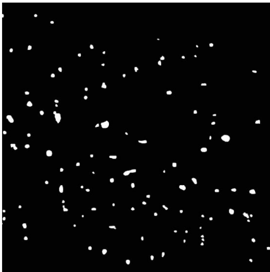
(b) High contrast image of the carbides and matrix.
