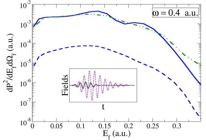
FIG. 7. The same as Fig. 6 for Al(100) and a carrier frequency  $\omega = 0.4$  a.u. BSB-V results neglecting the postcollision interaction, as explained in the text, are displayed with dot-dashed green line.
