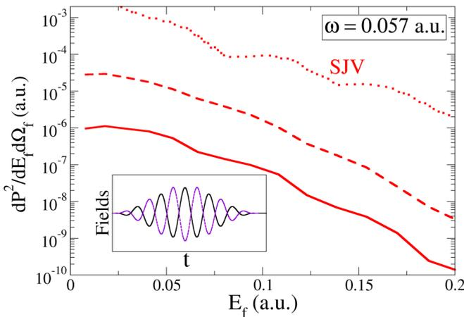
FIG. 6. PE distribution from Al(111) as a function of the final electron energy for a laser pulse with a carrier frequency  $\omega = 0.057$  a.u. The solid (dashed) red line shows BSB-V results with (without) the inclusion of the IS potential; the dotted red line shows SJV results from Ref. [17]. Inset: Corresponding laser and IS fields as a function of the time  $t$  are plotted with solid black and dashed violet lines, respectively.
