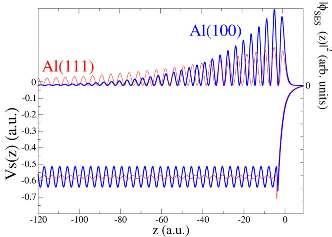
FIG. 2. Potential  $V_S(z)$  (lower graph), together with the square modulus of the corresponding SESs  $|\phi_{\text{SES}}(z)|^2$  (upper graph), with thick blue lines for Al(100) and thin red lines for Al(111).
