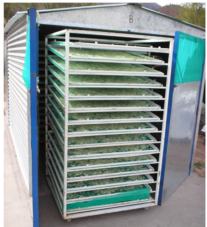
Fig. 4. Loading door of drying chamber, with carts and trays inside the chamber.
