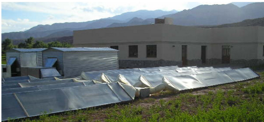
Fig. 2. Photograph of solar dryer. The collector array, fan cabinet and drying chamber are shown.
