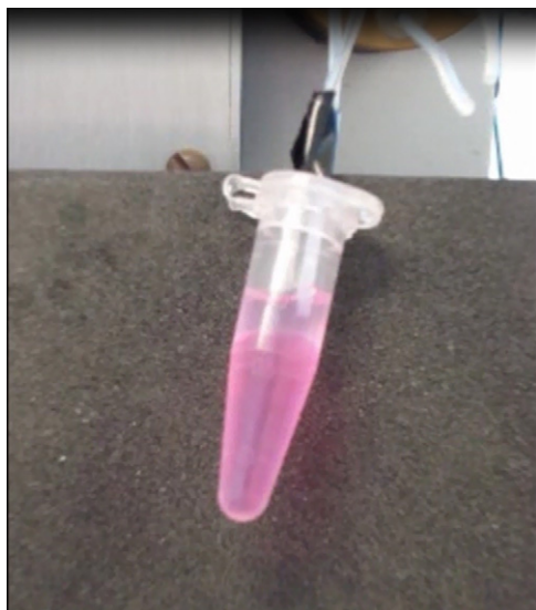
Fig. 3. Extraction procedure of sample solution measurement. The ion associate formed is extracted into the upper organic phase.
