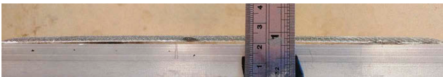
Figure 4a. Warpage almost disappeared after the post curing stage. Fabrics conditioned at 70% RH.
