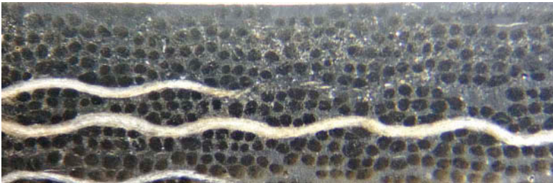
Figure 5b. Optical micrograph of C-50 showing a few amount of small pores.
