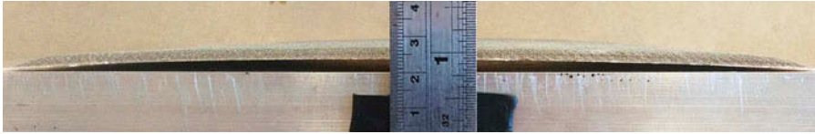
Figure 3b. Moderate warpage observed. Fabrics conditioned at 70% RH.
