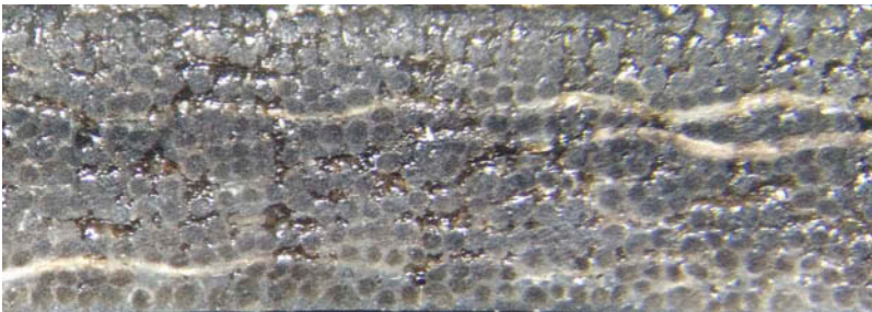
Figure 5c. Optical micrograph of C-90 showing a significant amount of large interconnected voids.
