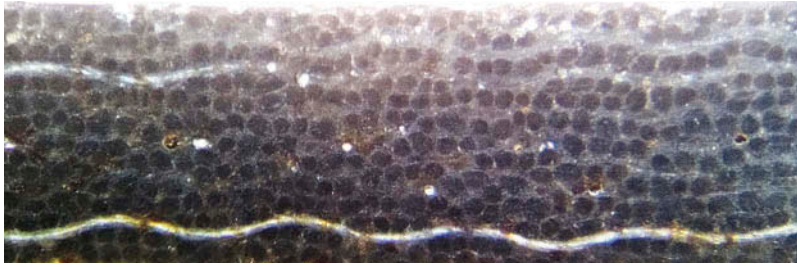
Figure 5a. Optical micrograph of C-D showing an almost void-free microstructure.
