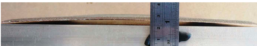
Figure 4b. Warpage decreased but still significant. Fabrics conditioned at 95% RH.
