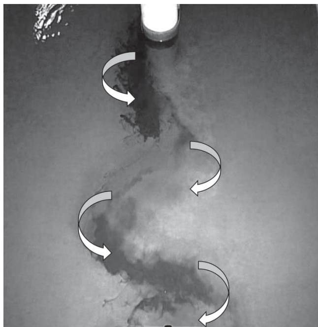
Figure 5 Visualization (using tracers) of coherent structures at the mixing interface of the confluence experimental configuration
