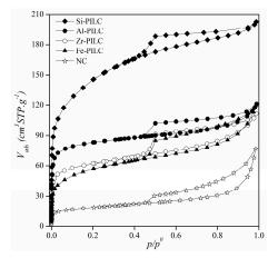
Figure 2. N<sub>2</sub> adsorption-desorption isotherms at 77 K for natural and pillared clay minerals.
