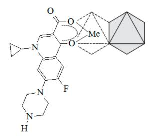
**Figure 8.** Representation of the structure proposed for the interaction between CPX<sup>-</sup> and atoms of metals on the PILC surface.
