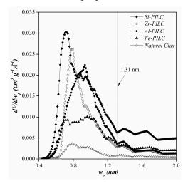
**Figure 3.** Pore side distribution of natural and pillared clay minerals where *V* is adsorbed volume and  $w_p$  is the pore size.
