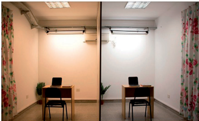
Figure 1 The experimental sets (warm and cool) at the higher level, with the wall lighting on (available in colour in online version)
