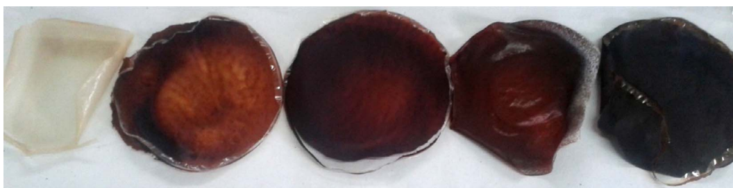
Fig. 1. Plasticized nanocomposite films. From left to right: 0, 2, 5, 7 and 10 wt.% MNP concentration.
