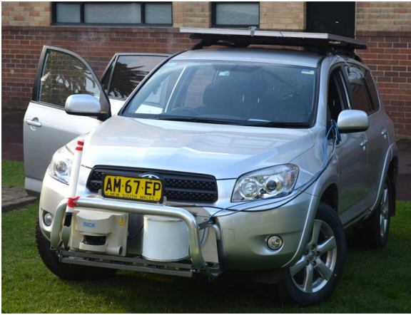
Fig. 3. Research vehicle equipped with multiple sensing modalities, including LIDAR, RADAR, GNSS and an inertial system (3-axis gyroscopes and accelerometers).
