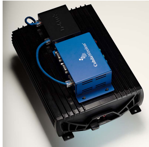
Fig. 4. Automotive computer including a gigabit switch, USB WiFi dongle and DSRC radio module. This hardware forms an easily deployed system for logging naturalistic driving data.
