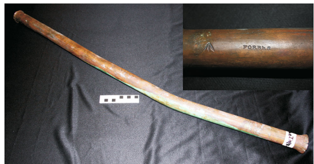
Fig. 1 HMS Impregnable bolt with a Forbes works stamp
