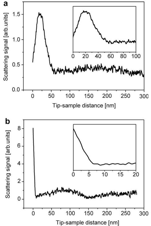
**Fig. 3.** Approach curves of the scattering signal at  $2\Omega$ . (a) 532 nm and (b) 633 nm incident wavelength (p-polarized). Curves have a clear dependence on the wavelength and show the signature of the field enhancement. The insets show enlarged scales for short distances.
