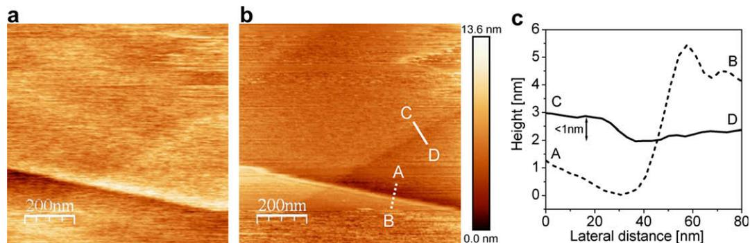
**Fig. 5.** (a) HOPG terraces recorded with the FESOM using NP-based probes and p-polarized 633 nm light. In (b) the STM topographic image is shown, with its color bar, for comparison and for the analysis of the heights. Lines marked in image (b) correspond to the profiles in (c). It can be seen that a subnanometer step is resolved in the optical image.
