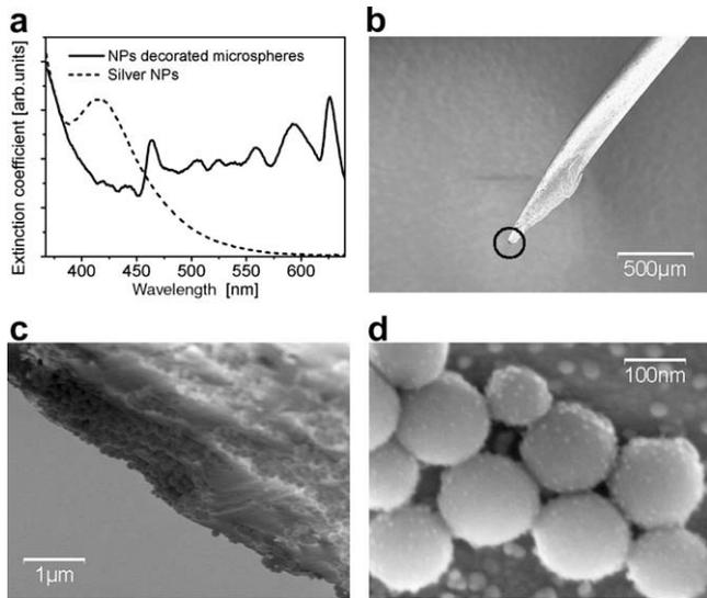
**Fig. 1.** The extinction spectrum of the colloidal solution of the NP-decorated microspheres is shown in (a). Multiple peaks in the spectrum reveal interaction between NPs. Non-interacting silver NPs spectrum is added for comparison. (b), (c) and (d) SEM images of the NP-based probes, with increasing resolution. Image (c) is the zoom of the circled zone in (b).
