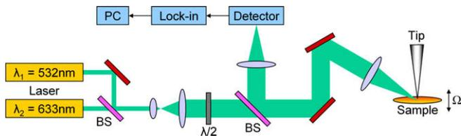
**Fig. 2.** Experimental setup scheme. The junction is illuminated from the side with a laser focused down to about 10 μm, which polarization can be controlled with a half waveplate. The sample is dithering at  $\Omega = 5$  kHz. The scattered light is collected in backscattering with the same optics and detected with a PIN photodiode. The lock-in detection is performed at  $2\Omega$ .
