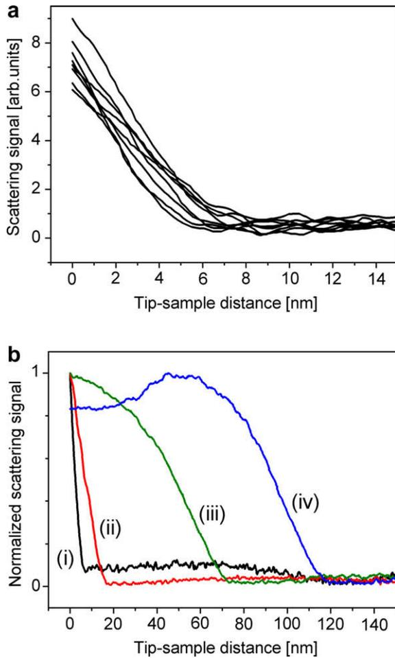
**Fig. 4.** Approach curves obtained on the first day are shown in (a). 633 nm incident light was used. The optical signal goes up at very short tip-sample distances. (b) Evolution of the approach curves during four days. From left to right: (i) first day, (ii) third day, (iii) and (iv) fourth day.
