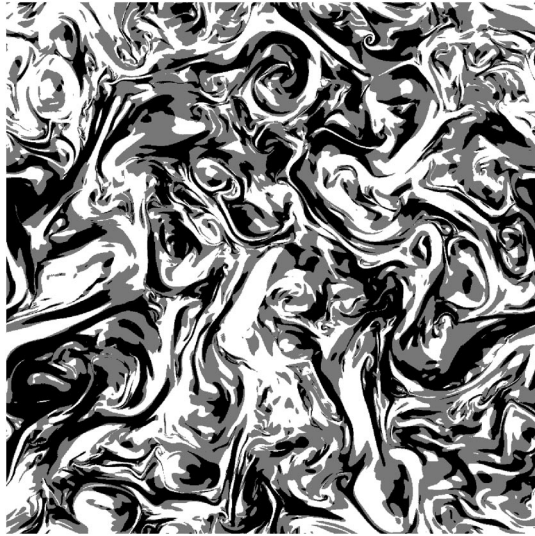
FIG. 6. Two-dimensional incompressible MHD simulation, showing areas where \cos\theta < -0.7 (black), |\cos\theta| < 0.7 (gray), and \cos\theta > 0.7 (white). Areas with highly aligned or antialigned velocity and magnetic field dominate the picture.
