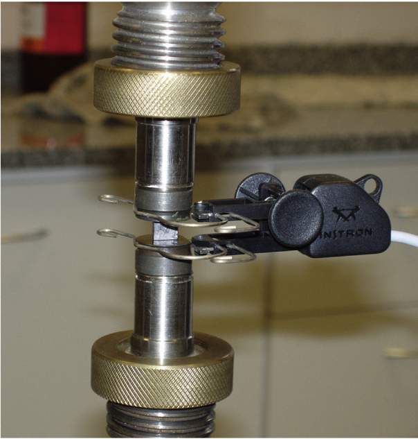
Fig. 3. A sample being compressed. The image shows how the extensometer was attached to measure the deformation.
