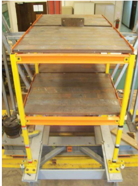
FIGURE 3 View of the added steel plates (color figure available online).
