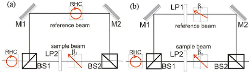
Fig. 1. Diagrams for the first (a) and second (b) experiment in the Mach-Zehnder interferometer analyzed in the text. Thin arrows (in red) represent the polarization state. BS<sub>i</sub>: Non polarizing beam splitters. LP<sub>i</sub>: Linear polarizers oriented at  $\beta_i$  with respect to the vertical.
