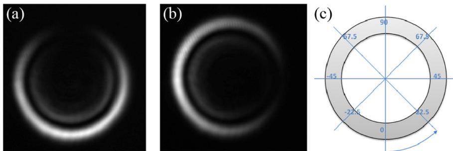
Fig. 7. Intensity distribution at the focal plane when a biaxial crystal is illuminated with linearly polarized light oriented (a) along the vertical, and (b) at  $-45^\circ$ . In (c) we indicate the orientation of the linearly polarized eigenpolarizations along the azimuth of the ring.
