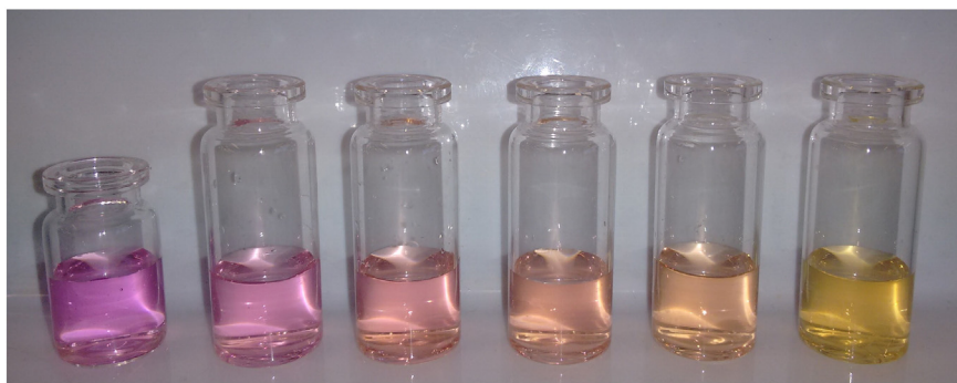
Fig. 5. Reaction of brightener in zinc electroplating bath with \text{MnO}_4^- . 150 \mu\text{l} of a 3.2 mM \text{KMnO}_4 solution was added to 5 ml of the standards and left to react for 15 min. Composition of the bath: see Table 1. From left to right: 0, 0.1, 0.3, 0.5, 0.7 and 0.9 ml/l (0, 1.13, 3.4, 5.7, 7.9 and 10.2 mM o-chlorobenzaldehyde).
