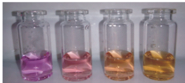
Fig. 2. Reaction of brightener in HCl\ 10^{-4} M solution with MnO_4^- . 150 \mu l of a 3.2 mM KMnO_4 solution (pH = 4 with HCl) was added to 5 ml of the standards and left to react for 10 min. From left to right: 0, 0.3, 0.5 and 0.7 ml/l brightener, equivalent to 0, 0.34, 0.57 and 0.79 mM in o-chlorobenzaldehyde, respectively.
