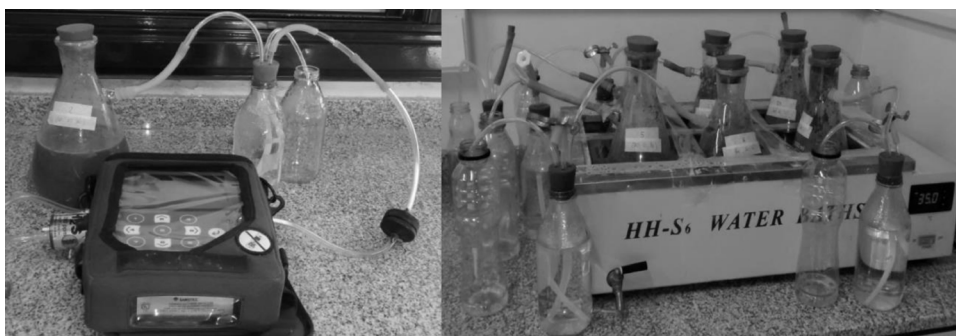
Fig. 1. Experimental arrangement; biogas and methane measurement.
