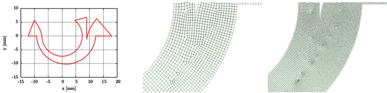
Fig. 3. Perimeter of the nozzle (left), original mesh (center), first refinement (right).
