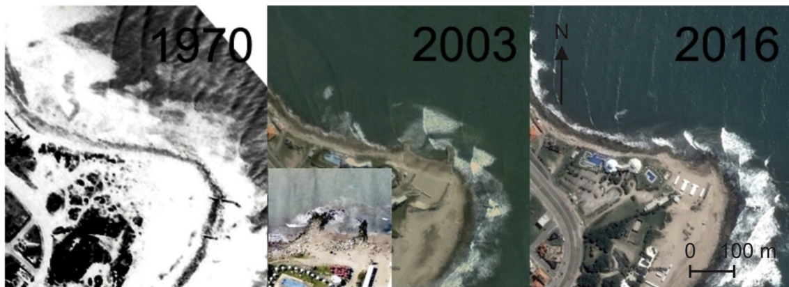
Fig. 8. Non-authorized groins were constructed at Punta Cantera, and later destroyed by the demand of Buenos Aires authorities.
