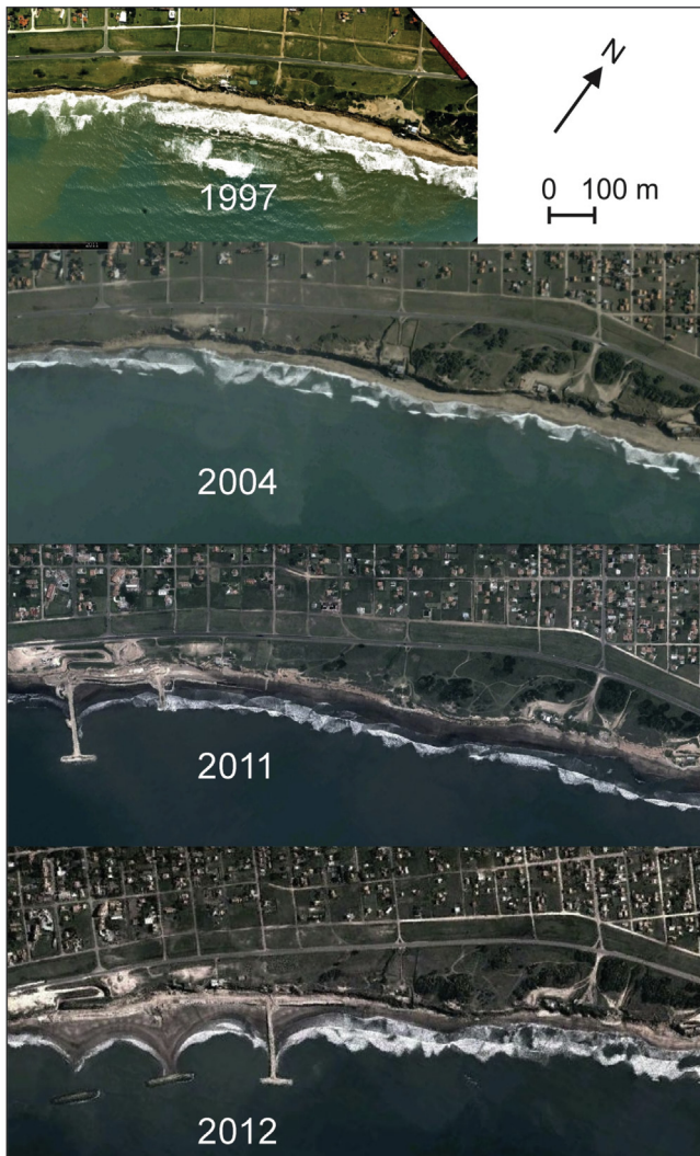
Fig. 6. Eight detached breakwaters were proposed in 2008. In 2012, the third breakwater (right) was not detached from the coast (modified from Isla, 2015).
