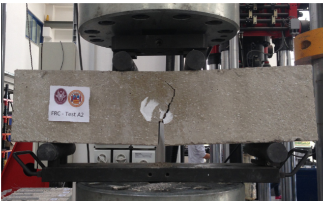
Fig. 8. Typical failure mode (HySP-FRC-0.75-0).
