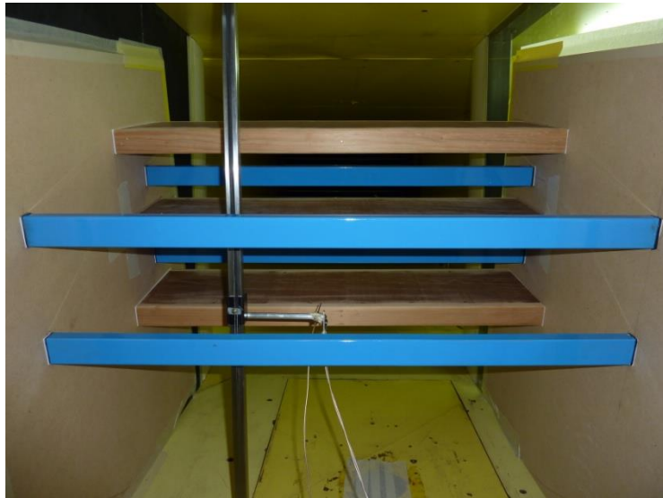
Fig. 3 Radar panels (wood), structure bars (blue) and vertical support of hot wire anemometer probe. View from downstream
