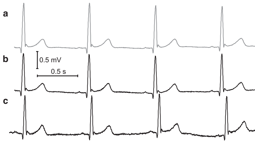
Fig. 5. ECG signals picked: (a) by standard disposable wet electrodes; (b) by the built capacitive electrodes placed on the skin; and (c) through a cotton T-shirt. Records in (a) and (b) were acquired simultaneously, and (c) corresponds to a different trial. Signal bandwidth was limited to 0.05–100 Hz and linear trends subtracted.
