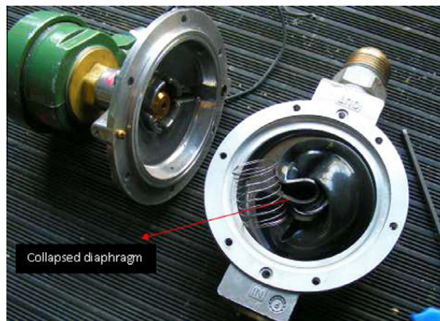
Fig. 10. Collapsed rubber diaphragm of solenoid valve.
