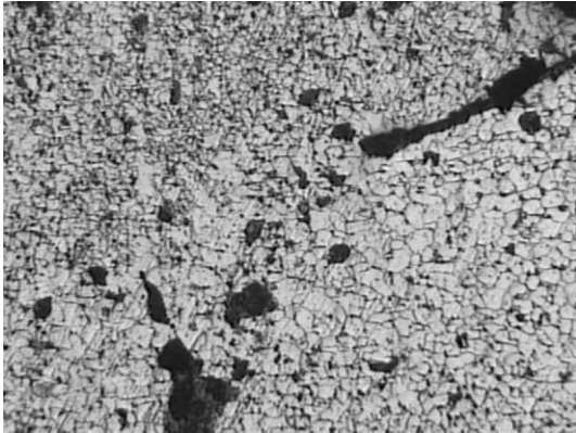
Fig. 5. Very sharp tips of defects ( \times 100 ).
