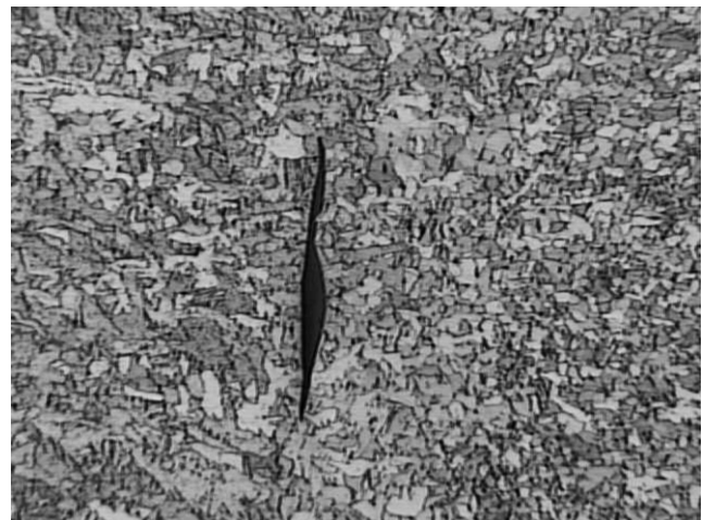
Fig. 12. A crack in the backing strip ( \times 100 ).
