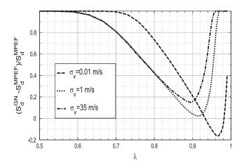
Fig. 4 Relative error between GN and MPFE for  $\sigma_{\eta} = 6$  and different velocity standard deviations
