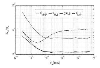
Fig. 6 Relative square root of the distance-MSE with respect to the standard deviation of velocity when  $\sigma_{\eta} = 3$  for MSE,  $d_{MLE}$ ; Linear Mean Square filter,  $d_{LMS}$ ; and Minimum Prediction Error Filtering,  $d_{MPFE}$
