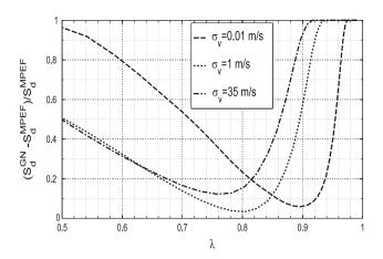
Fig. 2 Relative error between GN and MPFE for  $\sigma_{\eta} = 1$  and different velocity standard deviations
