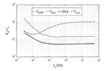
**Fig. 5** Relative square root of the distance-MSE with respect to the standard deviation of velocity when  $\sigma_{\eta} = 1$  for MLE, d<sub>MLE</sub>; Linear Mean Square filter, d<sub>LMS</sub>; and Minimum Prediction Error Filtering, d<sub>MPFE</sub>
