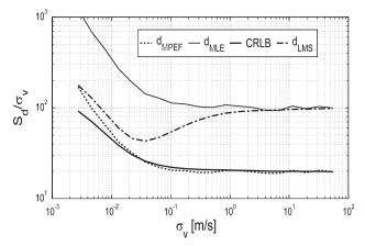
Fig. 7 Relative square root of the distance-MSE with respect to the standard deviation of velocity when  $\sigma_{\eta} = 6$  for MSE,  $d_{MLE}$ ; Linear Mean Square filter,  $d_{LMS}$ ; and Minimum Prediction Error Filtering,  $d_{MPFE}$
