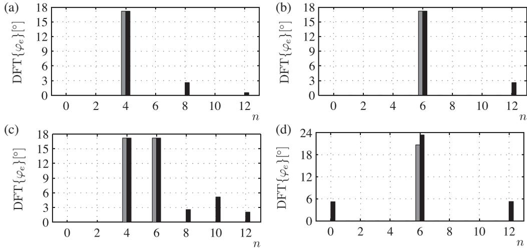
**Fig. 2.** Phase error harmonic distortion (Discrete Fourier Transforms of  $\varphi_e$ ). Error in estimated phase angle (black) and theoretical error (gray). Fundamental component and (a) a 30% of a 5th positive sequence harmonic, (b) a 30% of a 7th positive sequence harmonic, (c) a 30% of a 5th positive sequence harmonic and a 30% of a 7th positive sequence harmonic; and (d) a 30% of a 5th negative sequence harmonic and a 30% of a 7th positive sequence harmonic.
