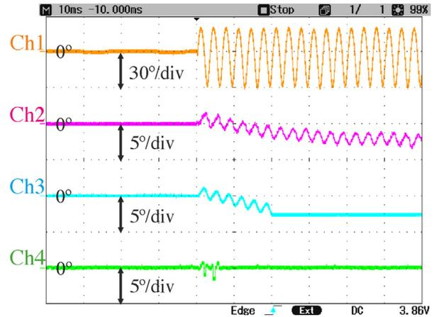
**Fig. 4.** Evaluation of phase error in several synchronized applications under 15% of the 5th negative sequence harmonic and 15% of the 7th positive sequence harmonic. (Ch1) Phase detector without filter stage, (Ch2) PLL proposed in [13], (Ch3) sequence detector proposed in [18] and (Ch4) fundamental positive sequence estimator proposed in [20].
