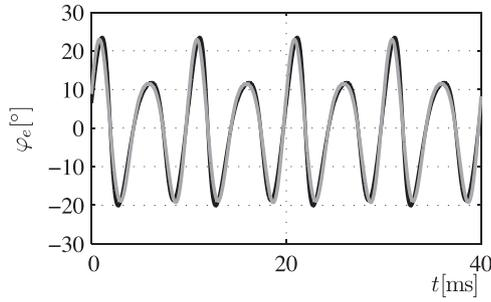
**Fig. 1.** Phase detector error (black) and theoretical error (gray) for a 30% of a 5th positive sequence harmonic and a 10% of a 7th positive sequence harmonic.
