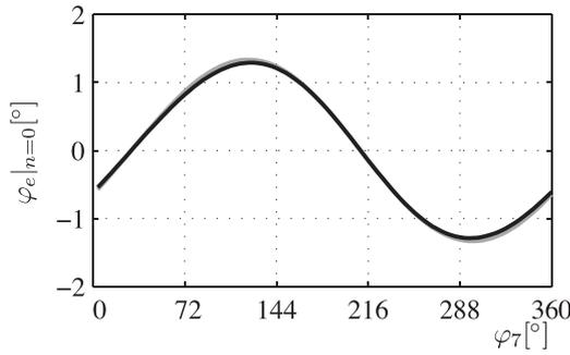
**Fig. 3.** Phase error in zero frequency ( $\varphi_e|_{n=0}$ ) implementing the phase detector (black) and Eq. (12) (gray).
