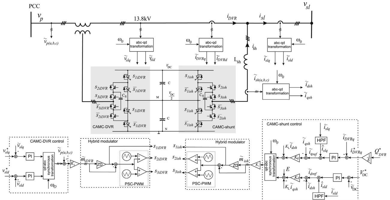
Fig. 3. Complete diagram of the control of the UPQC.
