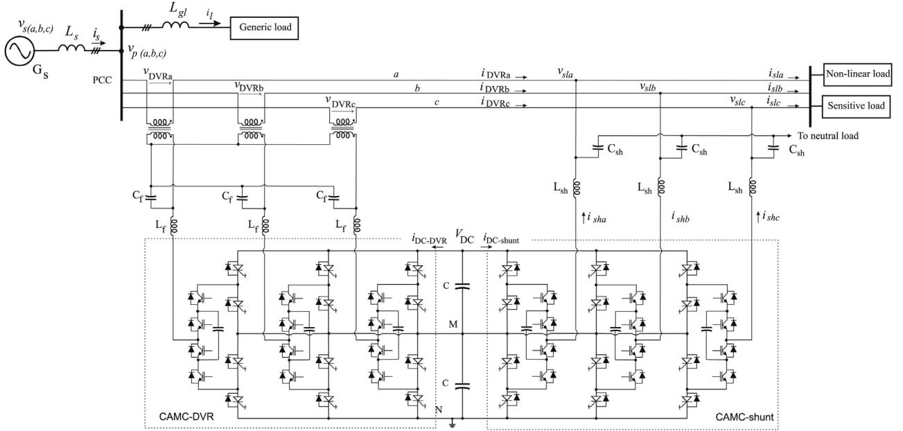
**Fig. 1.** A UPQC implemented with two back-to-back CAMCs.
