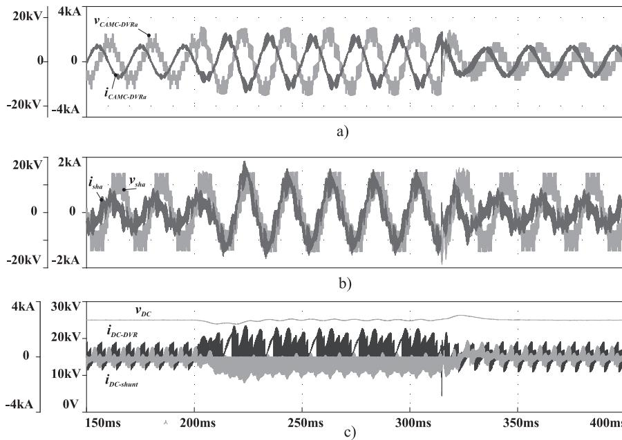
**Fig. 9.** (a) Output voltage and current of the CAMC-DVR, (b) output voltage and current of the CAMC-shunt and (c) DC currents in both side of the UPQC and DC voltage.
