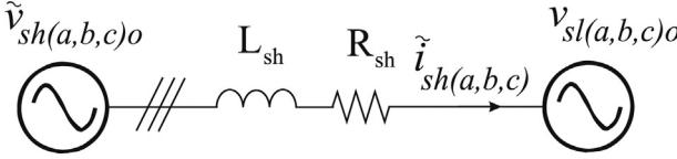
Fig. 4. Average dynamic model of the CAMC as a shunt compensator.
