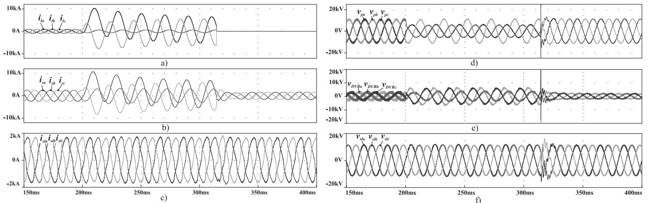
**Fig. 7.** Three phase currents and voltages in fault condition working. Currents on (a) the point of fault, (b) the voltage source and (c) the sensitive load. Voltages (d) in the PCC, (e) injected by the CAMC-DVR and (f) in the sensitive load.
