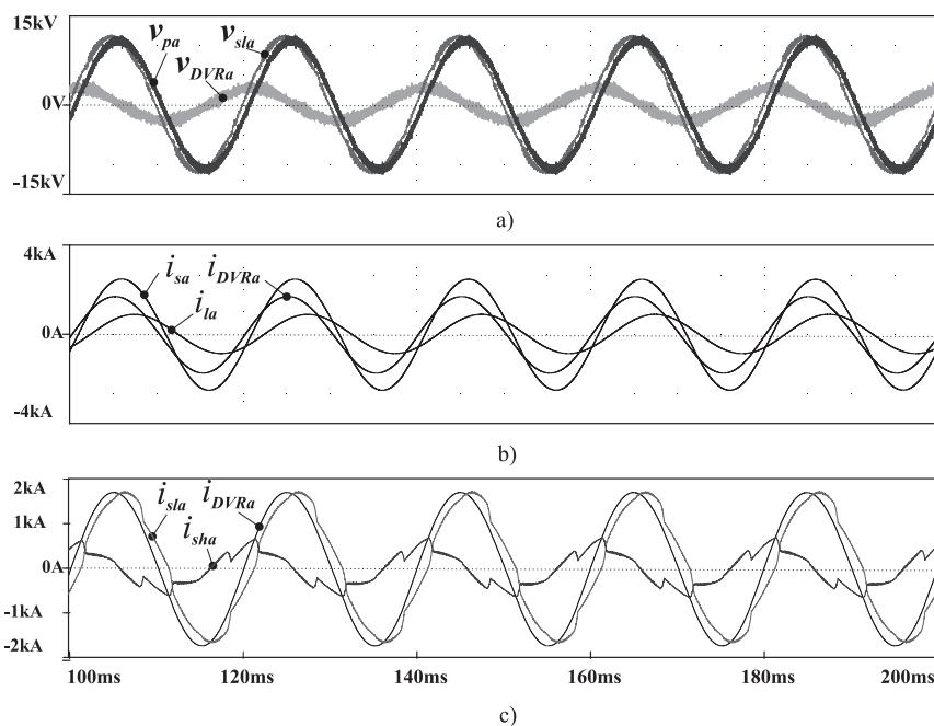
**Fig. 5.** Wave forms on phase-a for nominal working condition: (a) voltages, (b) currents on the PCC and (c) currents on the sensitive load connection point.
