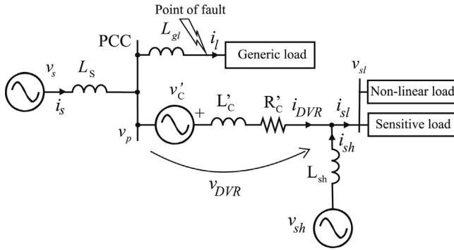
Fig. 2. Simplified single-line representation of the system.
