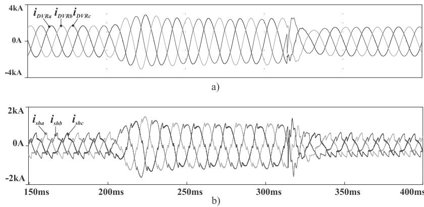
**Fig. 8.** Currents along the fault (a) on the CAMC-DVR and (b) on the CAMC-shunt.
