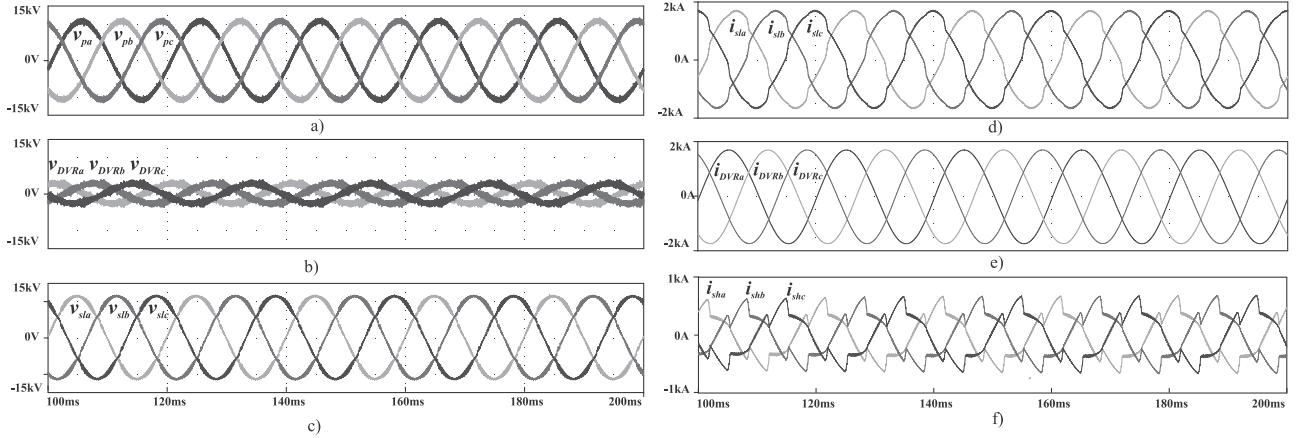
**Fig. 6.** Three phases voltages and currents in nominal condition working. Voltages in (a) the PCC, (b) injected by de CAMC-DVR and (c) the sensitive load. Currents on (d) the sensitive load, (e) CAMC-DVR and (f) CAMC-shunt.
