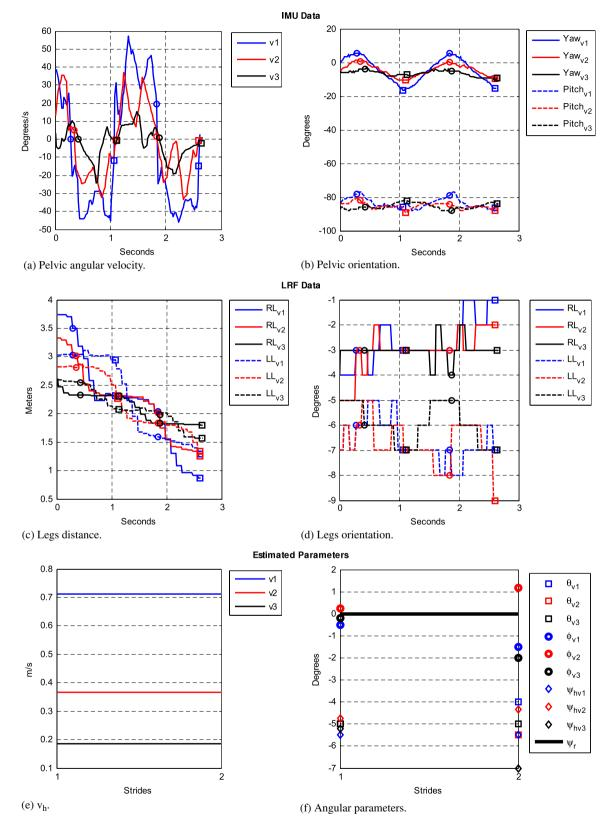
**Fig. 10.** Measurements and estimated parameters performed in the first experiment of the test of -5 degrees. (a) Pelvic angular velocities from *z*-axis gyroscope; (b) Pelvic orientation from IMU; (c) Legs distance curves from LRF detection; (d) Legs orientation curves from LRF detection; (e) Estimated  $v_h$ ; (f) Estimated  $\theta$ ,  $\psi_h$ ,  $\varphi$  and  $\psi_r$  angles.
