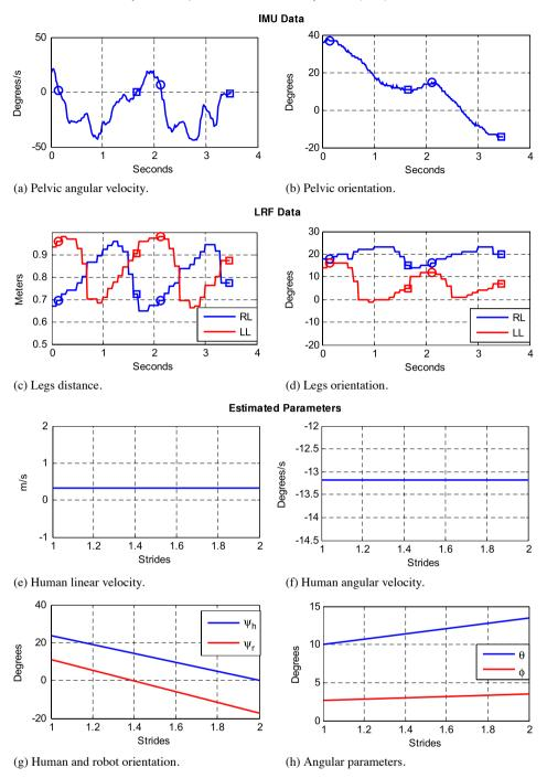
**Fig. 14.** Measurements and estimated parameters for  $v_h$  0.3 m/s and  $\omega_h$ -14°/s from the first experiment. (a) Pelvic angular velocity from *z*-axis gyroscope; (b) Pelvic orientation from the IMU; (c) Legs distance curves from LRF detection; (d) Legs orientation curves from LRF detection; (e) Estimated  $v_h$ ; (f) Estimated  $\omega_h$ ; (g) Estimated  $\psi_h$  and  $\psi_r$ ; (h) Estimated  $\theta$  and  $\varphi$  angles.
