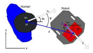
Fig. 2. Model for the human-robot interaction.
