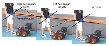
Fig. 4. External and internal measurement of the gait with the robot following the human in front.
