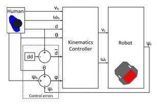
Fig. 3. Block diagram of the proposed controller.
