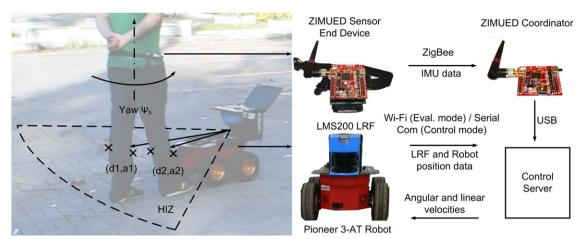
Fig. 5. Robot and sensor integration setup.
