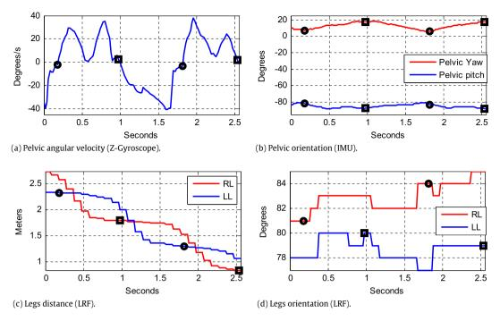
Fig. 6. Detection of zero crossing points over pelvic angular velocity.
