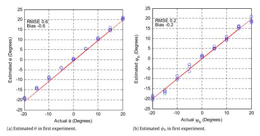
**Fig. 11.** Estimated values of  $\theta$  and  $\psi_h$  versus reference angles from the first experiment.
