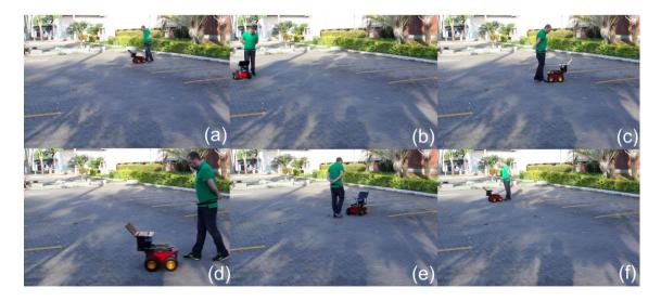
Fig. 18. Snapshots of the robot following in front experiment, performing an eight-shaped curve.
