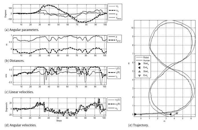
**Fig. 19.** Control data of robot following in front experiment performing an eight-shaped curve. (a) Angular parameters; (b) Distance parameters; (c) Linear velocities: control action  $v_r(C)$  and measured  $v_r(R)$  and  $v_h$ ; (d) Angular velocities: control action  $\omega_r(C)$ , and measured  $\omega_r(R)$  and  $\omega_h$ ; (e) Trajectory performed.
