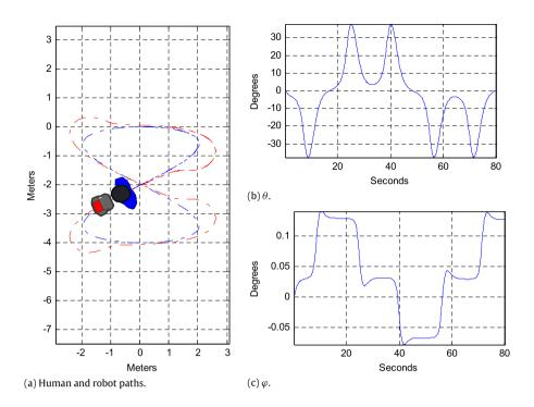
**Fig. 15.** Controller simulation. (a) Eight-shaped human path (blue dashed line), and the path of the robot following in front (red dashed line); (b)  $\theta$ ; and (c)  $\varphi$  responses. (For interpretation of the references to color in this figure legend, the reader is referred to the web version of this article.)
